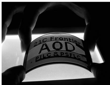
**Figure 11** 3'' plastic LCD sample using PILC mode.
