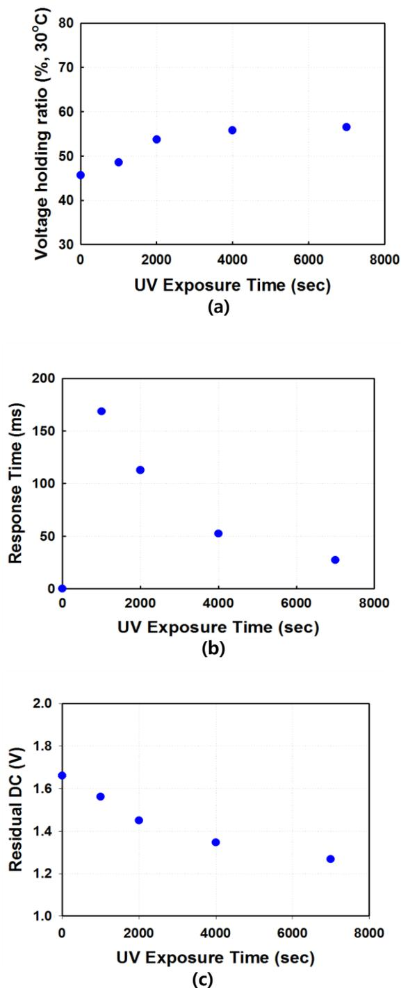
Figure 3. The measured during UV exposure time Capacitance characteristics of (a) VHR(voltage holding ratio), (b) RDC(residual direct current) (c) Response time.
