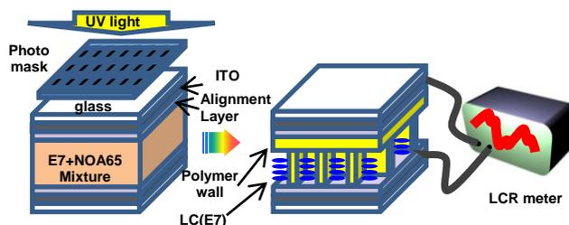
Figure 1. The capacitance were measured during UV exposure, simultaneously.
