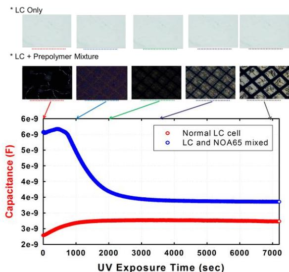
Figure 2. Microscopic Textures & Capacitance characteristics.
