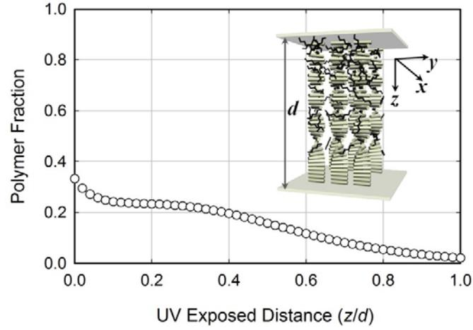
**Figure 1.** The volume fraction of the RM polymer with chirality and schematic diagram as function of the distance from UV illuminated surface. (Figure appears in color online.)
