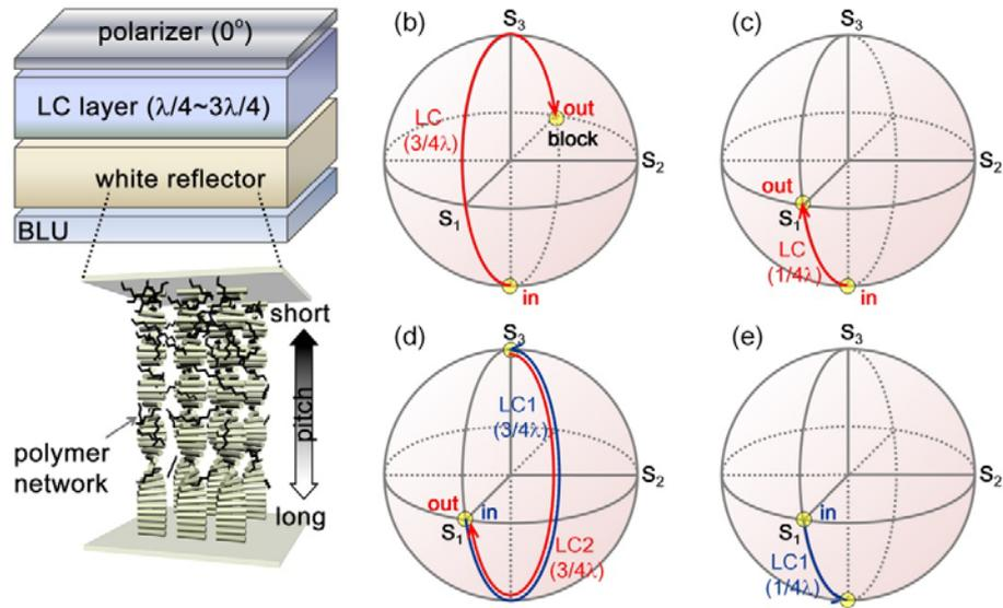
**Figure 3.** (a) Schematic diagram and (b)-(d) polarization representations of our proposed transfective LC display consisting of the nematic LC display as a conventional light modulator and the cholesteric white reflector as a transfective mirror. Optical pathways for (b) dark and (c) bright states in the transmissive mode, and for the (d) bright and (e) dark states in the reflective mode represented on the Poincaré Sphere. (Figure appears in color online.)
