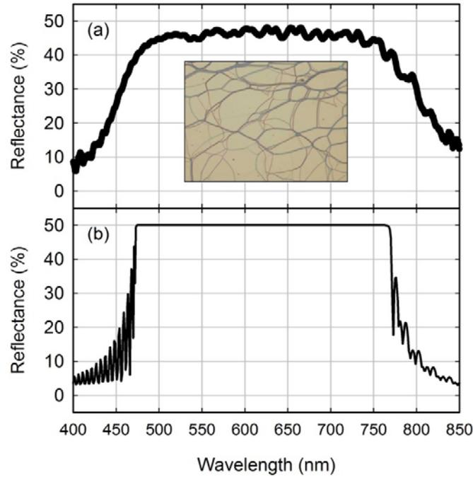
**Figure 2.** (a) Measured and (b) calculated spectra of reflection from the cholesteric white reflector. Inset image represents the reflected microscopic texture. (Figure appears in color online.)
