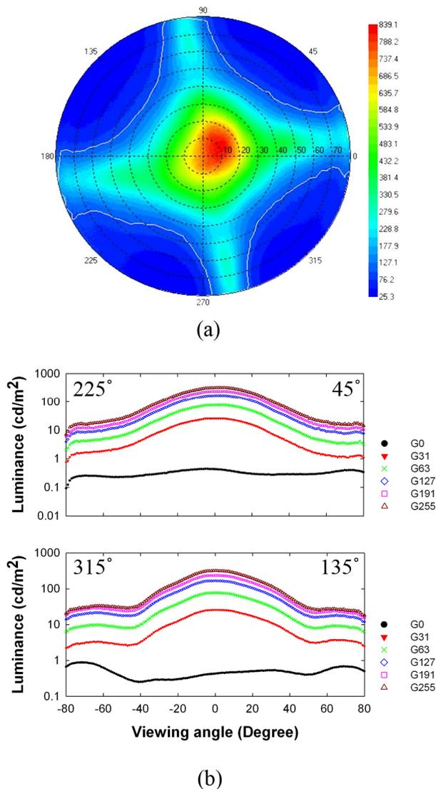
**Figure 4.** Viewing angle characteristics of fabricated 4.3-inch FFS mode panel using RM mixed alignment layer: (a) iso-contrast (white line was 100:1 of CR), (b) cross sectional luminance of each gray at the off axis, respectively
