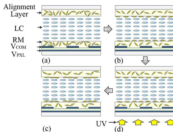
**Figure 1.** The schematic diagram of fabrication process of LC cell
