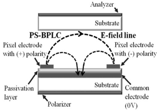
Figure 1. The schematic diagram of PS-BPLC device with an in-plane and fringe fields
