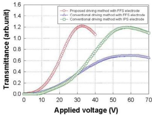
Figure 3. Measured voltage-transmittance curves
