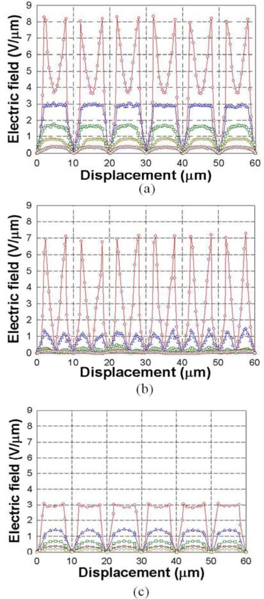
Figure 2. Electric field distributions according to the  $z/d$  where  $z$  is vertical position from the bottom substrate and  $d$  is the cell gap: (a) a proposed FFS cell, (b) conventional FFS and (c) conventional IPS cell
