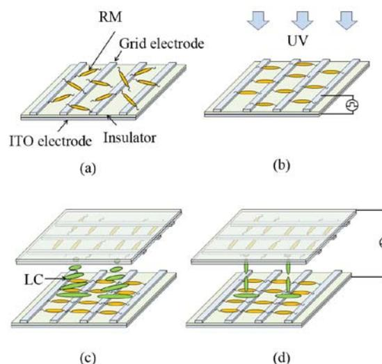
**Fig. 1** The schematic diagrams of the proposed aligning method: (a) randomly distributed RM on the FFS electrode and (b) uniformly aligned RM by the electric field and UV exposure. (c) White state and (d) black state in the TN cell.
