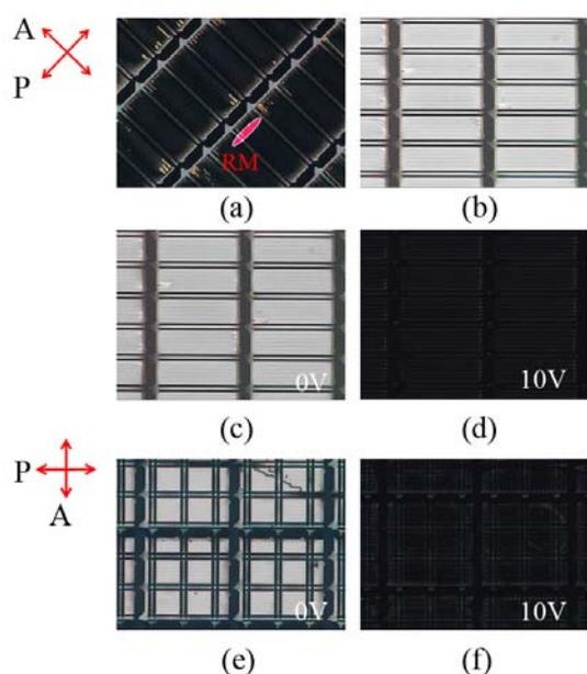
**Fig. 2** The microscopic textures of the planar cell (a) parallel and (b) rotated by  $45^\circ$  to the polarizer, the hybrid aligned cell (c) under no applied voltage and (d) under 10 V, and the TN cell (e) under no applied voltage and (f) under 10 V.
