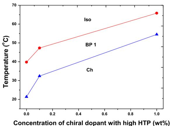
**Fig. 1** The plot of BP temperature range according to the concentration of the chiral dopant with high HTP
