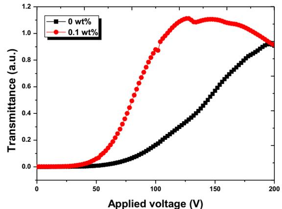
**Fig. 2** The plot of VT curves for the cell with 0 wt.% and 0.1 wt.% chiral dopant with high HTP
