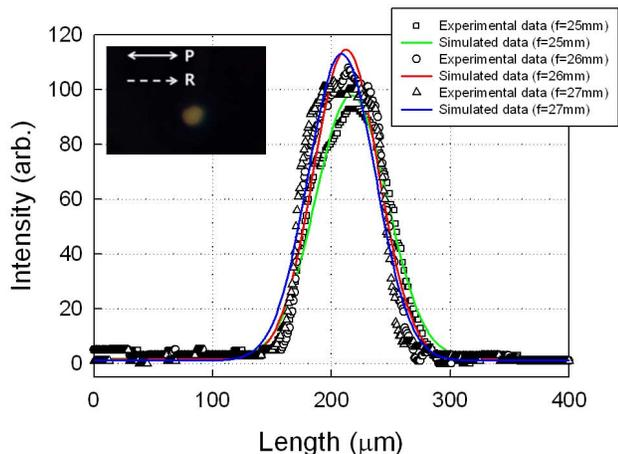
Figure 4. Focusing properties of the LCP Fresnel lenses: (a) the beam intensity profile of the lenses and (b) focused CCD images at focal point at 25mm
