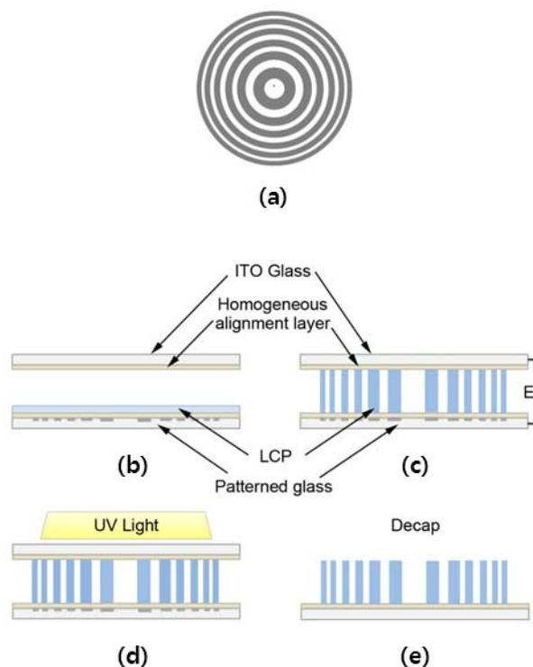
**Figure 1. The schematic diagram for fabricating a binary-phase Fresnel lens using the electrohydrodynamic instability (EHDI) of liquid crystalline polymer (LCP)**
