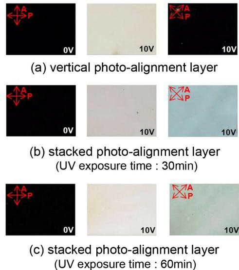
**Fig. 3** Microscopic textures of the ITN mode using photo-alignment method with (a) the only vertical photo-alignment layer, (b) the stacked photo-alignment layers exposed to NPUV for (b) 30 min and 60 min under crossed polarizers, respectively.
