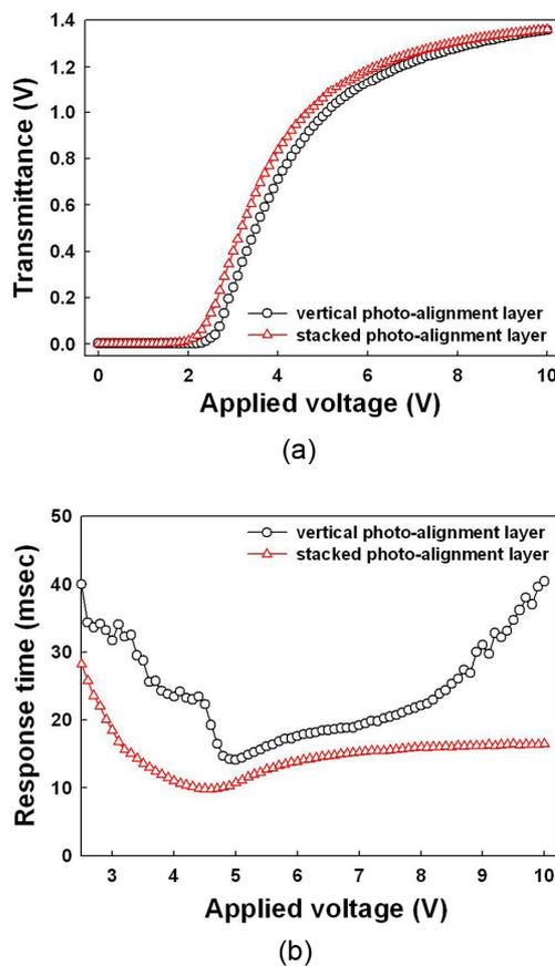
**Fig. 4 (a) The voltage-transmittance curve and (b) response time curve of two different layer systems with NPUV exposure for 60 min.**
