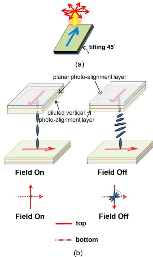
**Fig. 2** The schematic diagrams of (a) our UV exposure condition and (b) the ITN mode with applying voltage.
