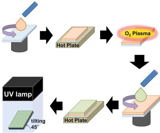
**Fig. 1** The schematic diagrams of fabrication process.
