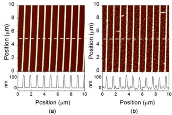
**Fig. 2** The AFM images of (a) the line pattern nano-scale structures on cPVP layer (b) the pentacene layer on it with nano-scale structures. The profiles represent the surface morphologies depicted by the dash lines in each AFM image.
