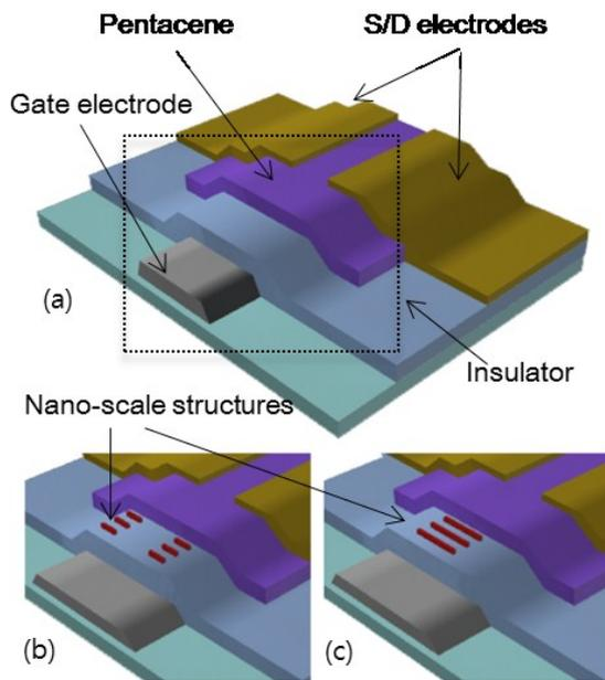
**Fig. 1** Schematic diagram of OTFTs with (a) no line patterns and [(b), (c)] nano-scale structures are formed at (b) S/D regions, (c) channel region, respectively
