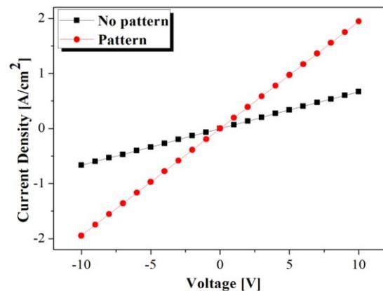
**Fig. 3** Current density characteristics on top Au electrode depending on applied voltage for bottom-Au/pentacene/top-Au structure.
