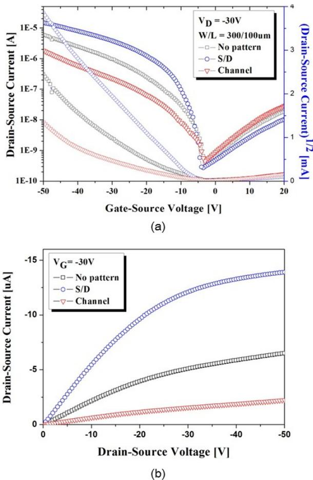
**Fig. 4 Electrical characteristics of OTFTs with/without no line patterns, (a) transfer curves at  $V_D = -30V$ , (b) output curves at a  $V_G = -30V$**
