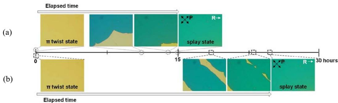
**Fig. 2.** The changed transmittance as the elapsed time of  $\pi$  twist state in designated pixel area measured by POM: (a) conventional BCSN LC cell and (b) BCSN LC cell by the surface treatment.
