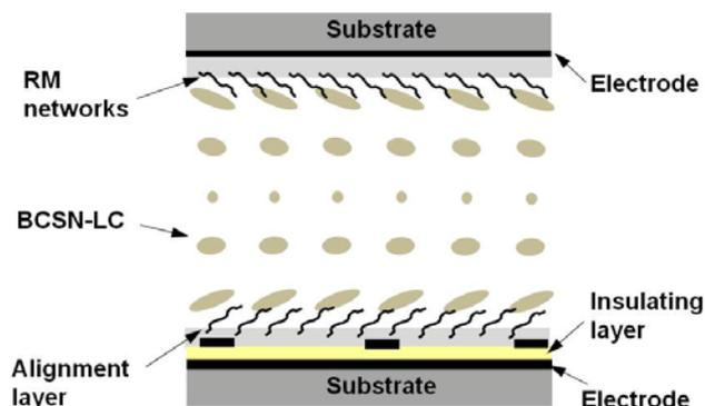
**Fig. 1. The schematic diagram of the cross section of the BCSN-LC cell structure by the surface treatment proposed in this work.**
