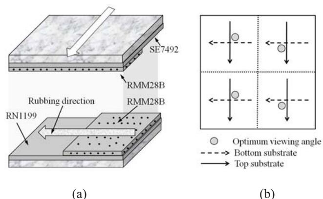
**Fig. 1. Schematic diagram of DDTN LC cell proposed in this work: (a) the cross-section and (b) direction of pre-tilt angle and optimum viewing angle in respective sub-pixels**
