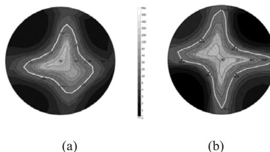
**Fig. 3. Viewing angle characteristics of (a) single-domain TN mode and (b) DDTN mode proposed in this work.**
