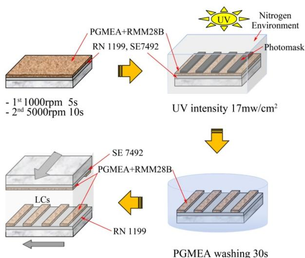
**Fig. 2. The schematic diagram of fabrication progress for DDTN LC cell proposed in this work.**
