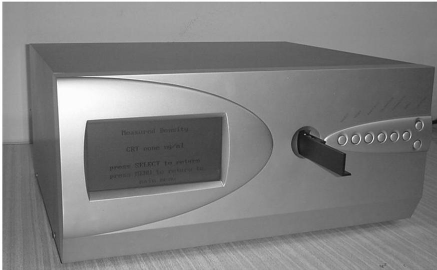
Figure 2. The 1D fluorescence scanner. The width is 37cm.
