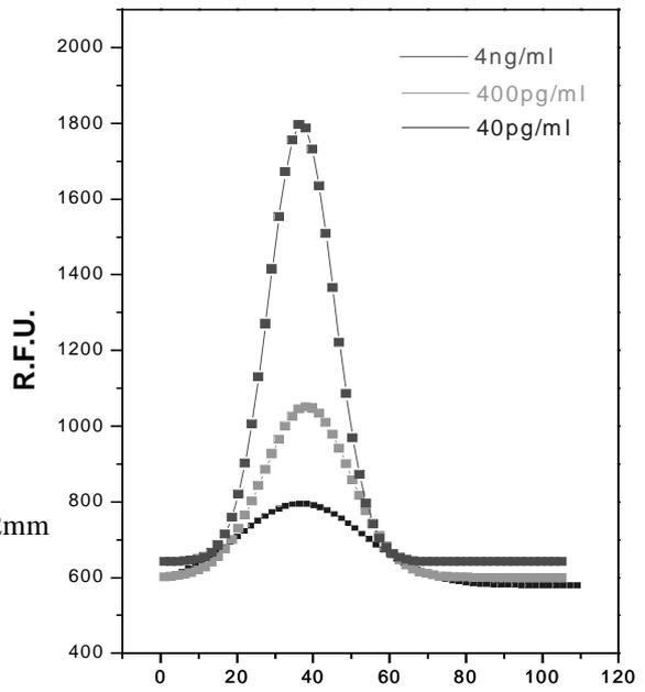
Figure 4. Comparison of signal for differing densities of the Prostate Specific Antigen (PSA). The ordinate is in arbitrary unit.
