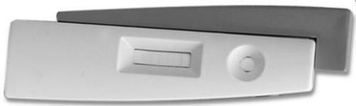
Figure 3. The sample cassette. The strip in the middle was 12mm long.
