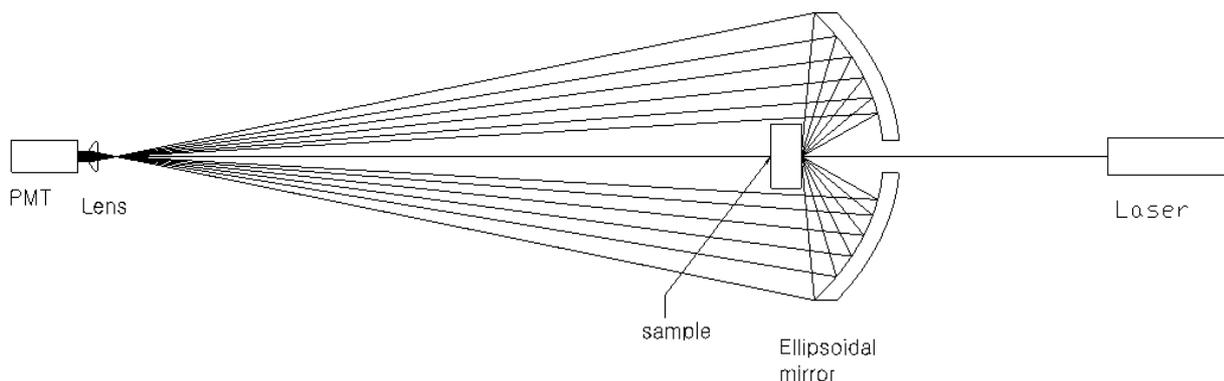
Figure 1. Optical layout of the system.
