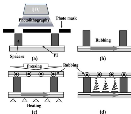
**Figure 1** The schematic diagrams of our simple process: (a) coating SU-8 on PI layer by UV photolithography, (b) rubbing in definite directions, (c) assembling top and bottom with heating and pressing, and (d) filling the fabricated cell with TN LC
