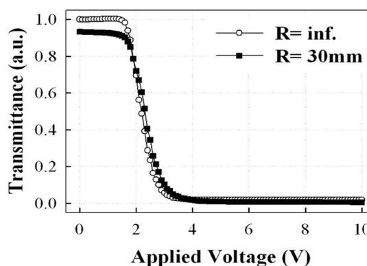
**Figure 3** The EO characteristic of a suggested TN cell depends on degree of bending
