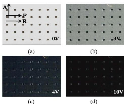
**Figure 2** Microscopic photographs of the TN mode fabricated with the adhesive patterned spacers at (a) 0V, (b) 3V, (c) 4V, and (d) 10V. Here, R, A, and p are a rubbing direction of bottom substrate, a direction of the upper analyzer, and a direction of lower polarizer, respectively
