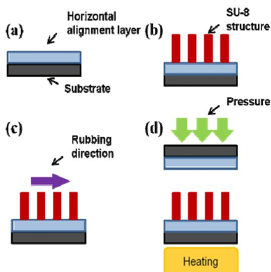
**Figure 1.** The fabrication process; (a) coating planar alignment layer on substrates, (b) forming the patterned spacers with SU-8, (c) rubbing the substrate, and (d) assembling two substrates under heating and pressing
