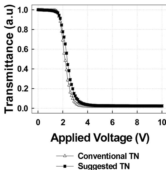
Figure 3. EO curves of the conventional TN LC cell and our TN LC cell fabricated with the adhesive patterned spacers.
