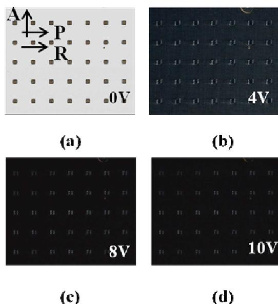
Figure 2. Microscopic photographs of the TN mode fabricated with the adhesive patterned spacers at (a) 0 V, (b) 4 V, (c) 8 V, and (d) 10 V. Here,  $R$ ,  $A$ , and  $P$  are a rubbing direction of bottom substrate, a direction of the upper analyzer, and a direction of the lower polarizer, respectively.
