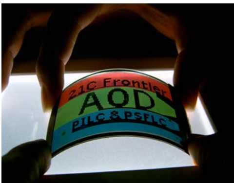
Fig 10 3-inch size LC sample using plastic substrates with pixel-isolated liquid crystal structure
