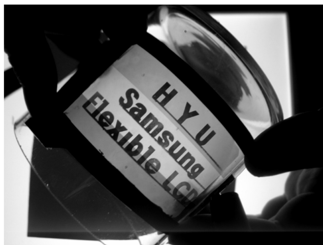
Figure 5. The photograph of prototype 3 inch plastic LCD using the proposed technique.
