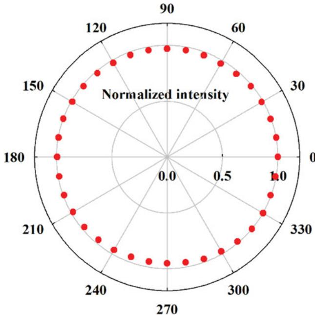
**Figure 5.** Normalized intensity of the proposed MLA at the focal point as a function of the polarization state of incident light.
