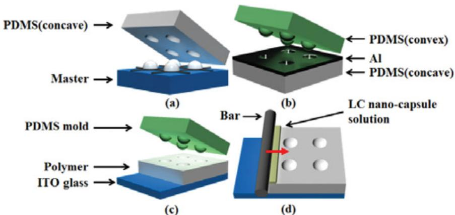
**Figure 2.** Schematic diagram of fabrication procedure. (a) Transferring master substrate to PDMS. (b) Transferring concave PDMS with aluminum layer to convex PDMS. (c) Stamping LCP lens structure on an ITO glass substrate with PDMS mold. (d) Bar coating LC nano-capsule solution on the LCP lens structure.
