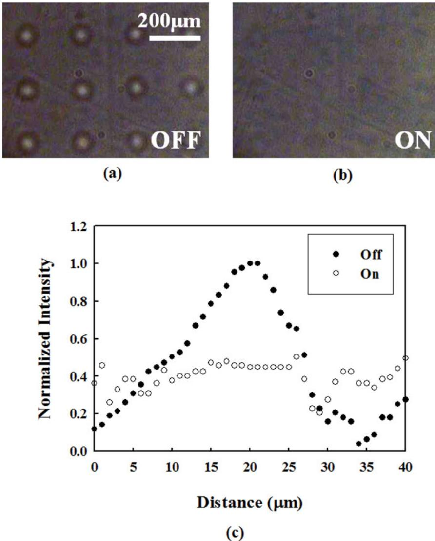
**Figure 4.** Microscopic images of (a) focused beam pattern without applied electric field, and (b) with applied electric field. (c) Spatial light intensity profiles.
