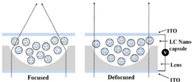
Figure 1. Operating principle for the proposed isotropic MLA.
