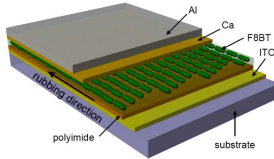
Fig. 1. Schematic diagram of the linearly polarized light emitting device proposed here.
