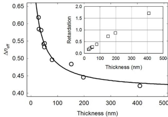
Fig. 2. The effective optical birefringence ( $\Delta n_{\text{eff}}$ ) and measured optical retardation (inset) of the F8BT film as a function of thickness. The solid curve depicts the least square fit to Eq. (1).
