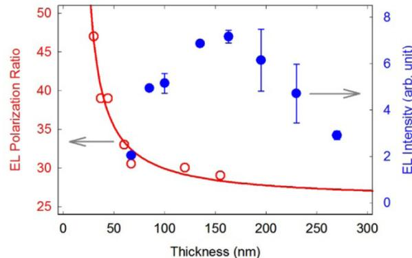
Fig. 4. The EL polarization ratio and the EL intensity of the F8BT-based OLEDs as a function of thickness. The solid curve depicts the least square fits to Eq. (4).
