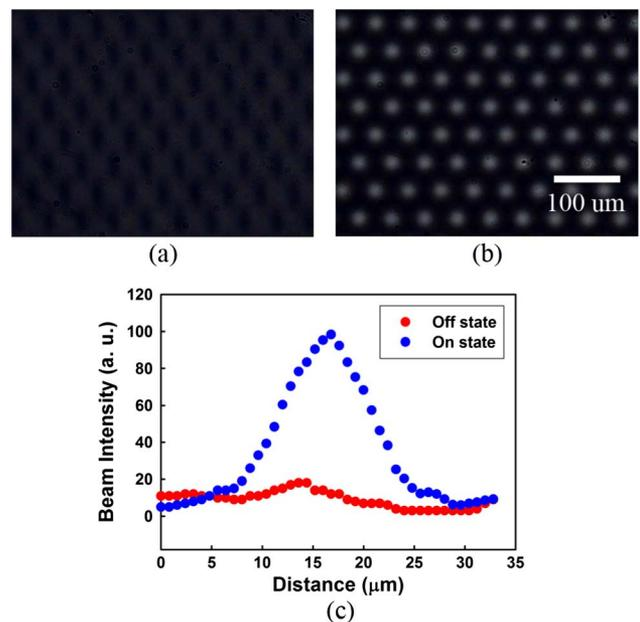
Fig. 5. Microscopic images of focused beam patterns at (a) 28°C and (b) 45°C. (c) Spatial light intensity profiles at the focal plane.
