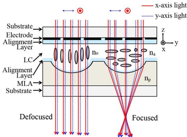
Fig. 1. Operating principle for the proposed MLA system.
