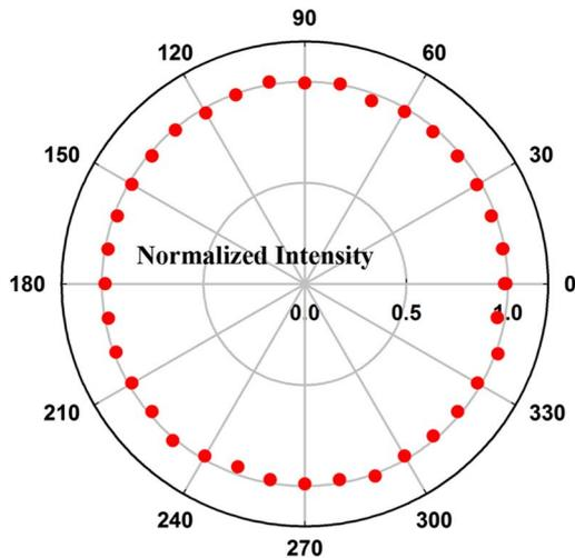
Fig. 6. Normalized beam intensity of the proposed MLA at the focal point as a function of the polarization state of incident light.
