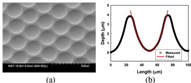
Fig. 2. SEM image and surface profile of an MLA structure.
