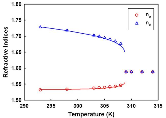
Fig. 4. Temperature-dependent refractive indices of 5CB LC at a wavelength of 589 nm. Triangles and circles represent experimental data, and solid lines were fit using the Wu model.
