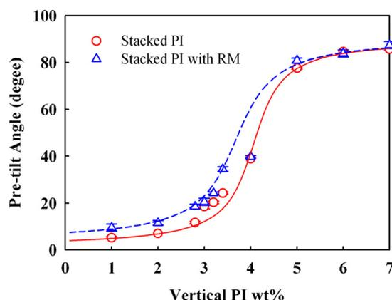
FIG. 5. Pretilt angle as a function of vertical alignment layer concentration.
