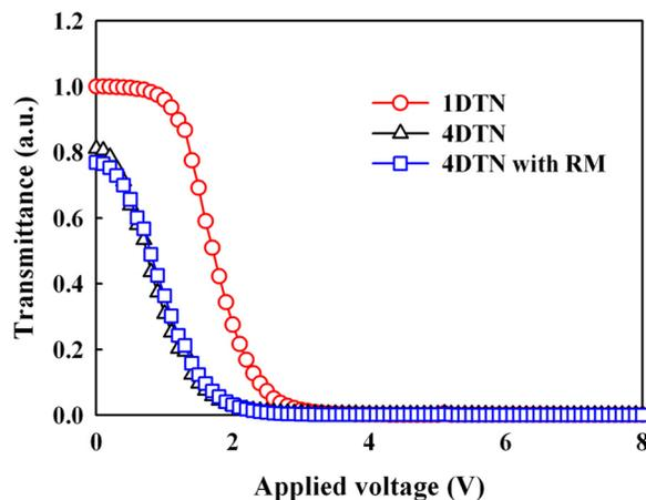
FIG. 7. Transmittance characteristics as a function of applied voltage for 1D TN and 4D TN with or without RM cells.
