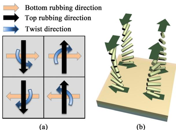
FIG. 1. (a) Rubbing and twist directions for each sub-pixel of the 4-D TN structure. (b) Schematic view of the liquid crystal molecule configuration of each sub-pixel.
