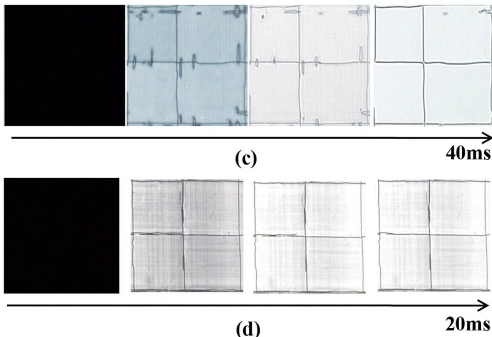
FIG. 8. (a) Rise and (b) fall characteristics for 1D TN and 4D TN cells with or without RM. Time resolved textures for 4D TN cells (c) without RM and (d) with RM.
