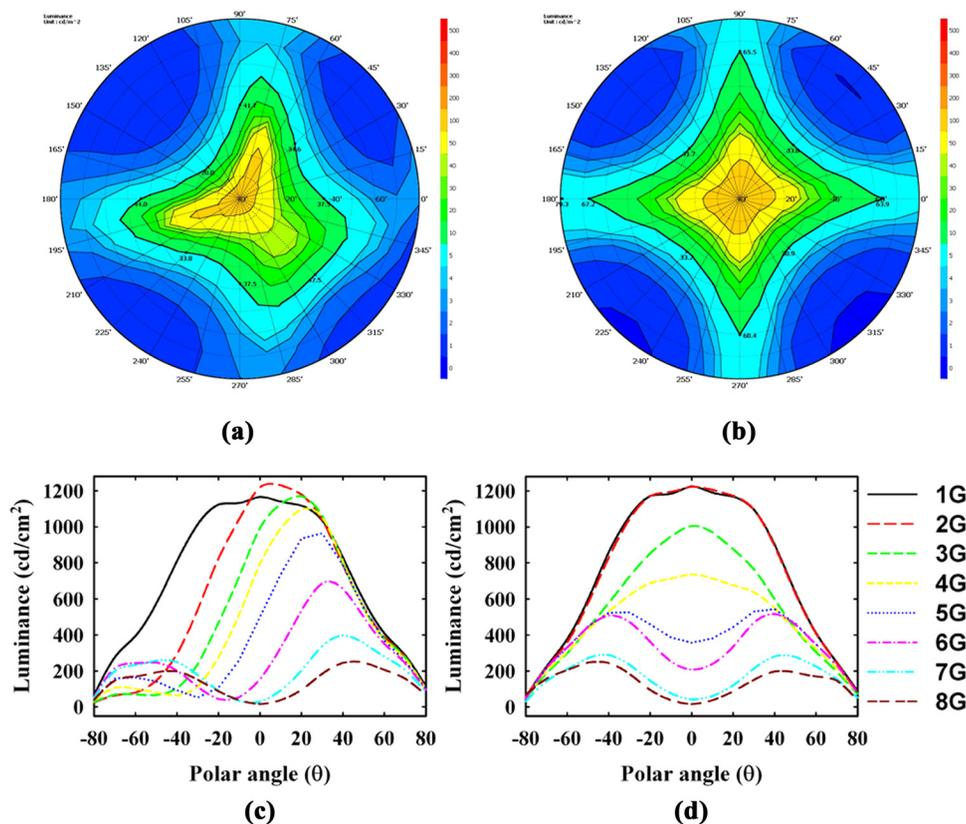
FIG. 3. Iso-contrast map of a (a) conventional 1-D TN cell and (b) stable 4-D TN cell. Gray inversion characteristics of (c) conventional mono-domain TN cells and (d) stable 4-D TN cells.
