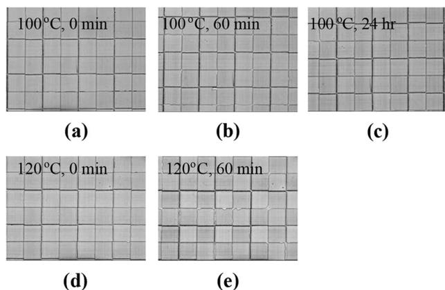
FIG. 6. Thermal stability of a 4-D TN sample with an RM mixed vertical alignment layer of 2.8 wt. %.
