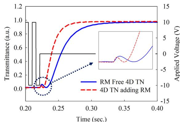
FIG. 9. Response time characteristics of conventional (RM free) 4D TN and RM added 4D TN.
