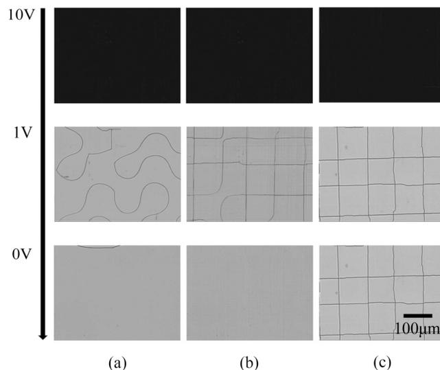
FIG. 2. Images of the 4-D TN structure at pretilt angles of (a) 4°, (b) 7°, and (c) 18°.
