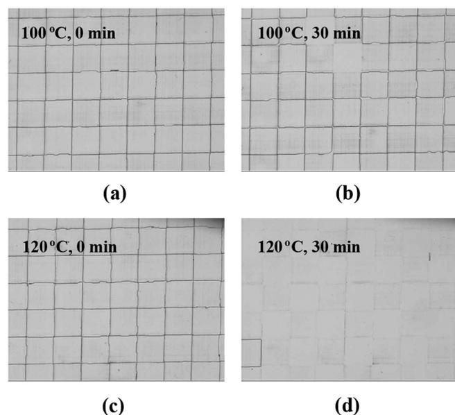
FIG. 4. Thermal stability of a 4-D TN cell with an 18° pretilt angle.
