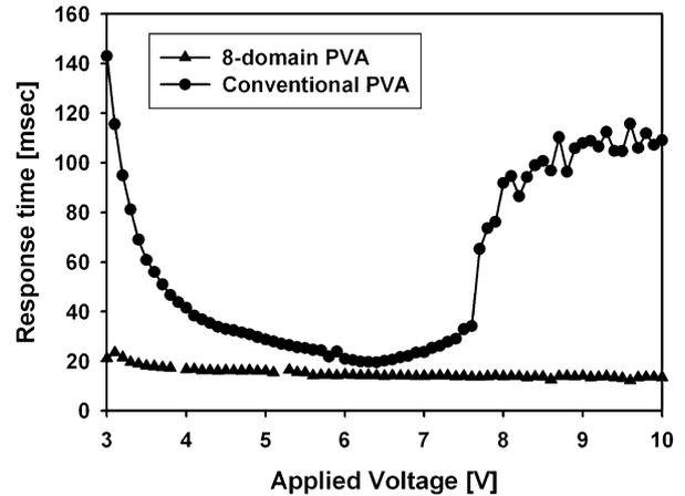
Fig. 5. Response time characteristics of the conventional PVA mode and our advanced PVA mode.
