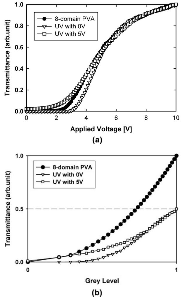
**Fig. 3.** (a) The voltage–transmittance characteristics and (b) the grey–transmittance characteristics with gamma-correction of  $\gamma = 2.2$ .
