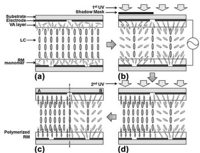
Fig. 1. The schematic diagram of our advanced SC-PVA mode and the fabrication processes.
