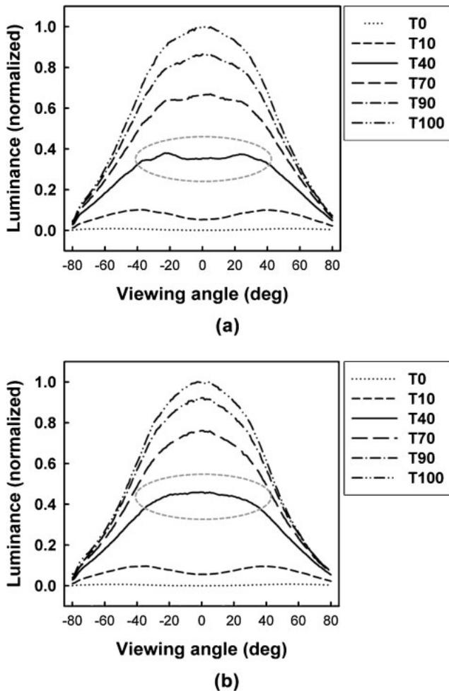
Fig. 4. Comparison of brightness viewing characteristics between (a) a conventional four-domain PVA mode and (b) the advanced eight-domain PVA mode for 45° with respect to polarizers.
