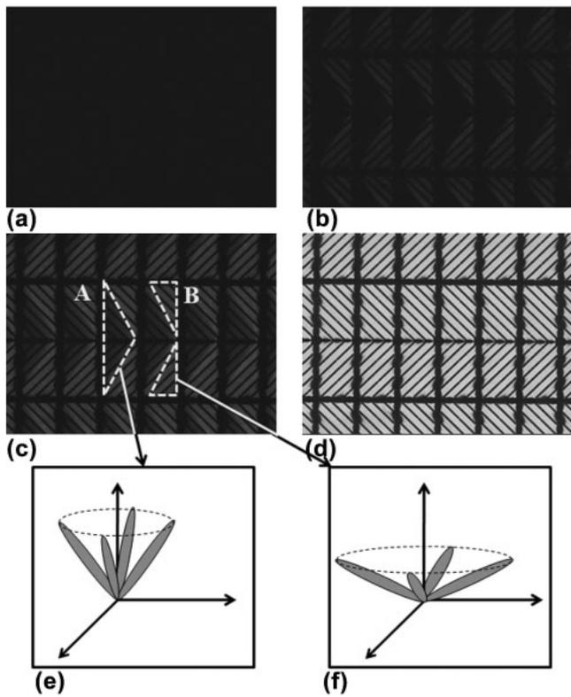
**Fig. 2.** Microscopic textures under crossed polarizers with (a) 0, (b) 3.2, (c) 4.5, and (d) 10 V, respectively. Schematic diagrams of LC directors with an applied voltage for area (e) A and (f) B, respectively.
