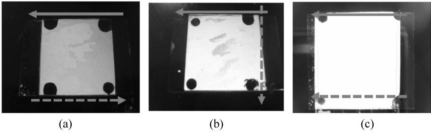
**FIGURE 4** The textures of samples under crossed polarizers with different direction of LC injection with respect to the rubbing direction. The solid and dotted lines indicate LC injection and rubbing direction, respectively.
