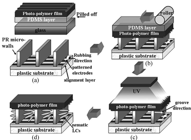
**FIGURE 2** Fabrication of the proposed plastic LCD with a single substrate by laminating the cover film. (a) Preparation of the photo-polymer film and the bottom plastic substrate with polymer walls (b) Laminating process by soft roller (c) UV irradiation for solidification and tight bonding of cover film after removing the TN layer (d) LC injection and resultant single substrate flexible TN LC cell.
