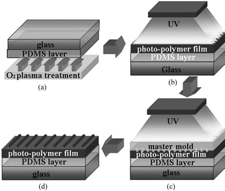
**FIGURE 1** The schematic diagram for the fabrication of the UV curable photo-polymer cover film on the supporting layer. (a)  $O_2$  plasma treatment on the spin-coated PDMS layer (b) Spin-coating and partial UV curing of photo-polymer film (c) Stamping of master mold on the photo-polymer film and UV curing (d) Resultant structure of photo-polymer with micro-grooves.
