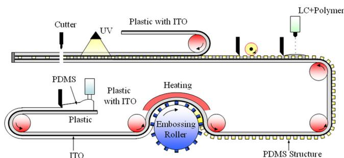
FIGURE 12 — Schematic diagram of continuous roll processing for the fabrication of plastic LCDs using the methods presented here.
