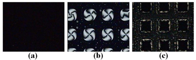
**FIGURE 7** — Polarizing optical microscopic images of PILC cell where the phase separation is induced by surface wetting properties of LC and polymer on the patterned alignment layer. Before UV exposure, (a) and (b) are obtained in the absence and presence of an applied voltage, respectively. (c) is obtained in the absence of an applied voltage after UV exposure.
