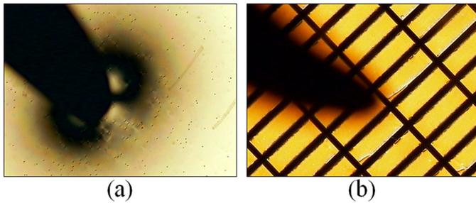
**FIGURE 8** — Alignment textures of (a) a normal sample and (b) a PILC sample fabricated using the plastic substrates. The polarizing microscopic textures were taken in the presence of an external point pressure with a sharp tip.
