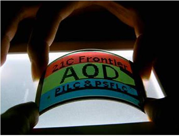
FIGURE 11 — A 3-in. plastic LCD sample in the PILC mode.
