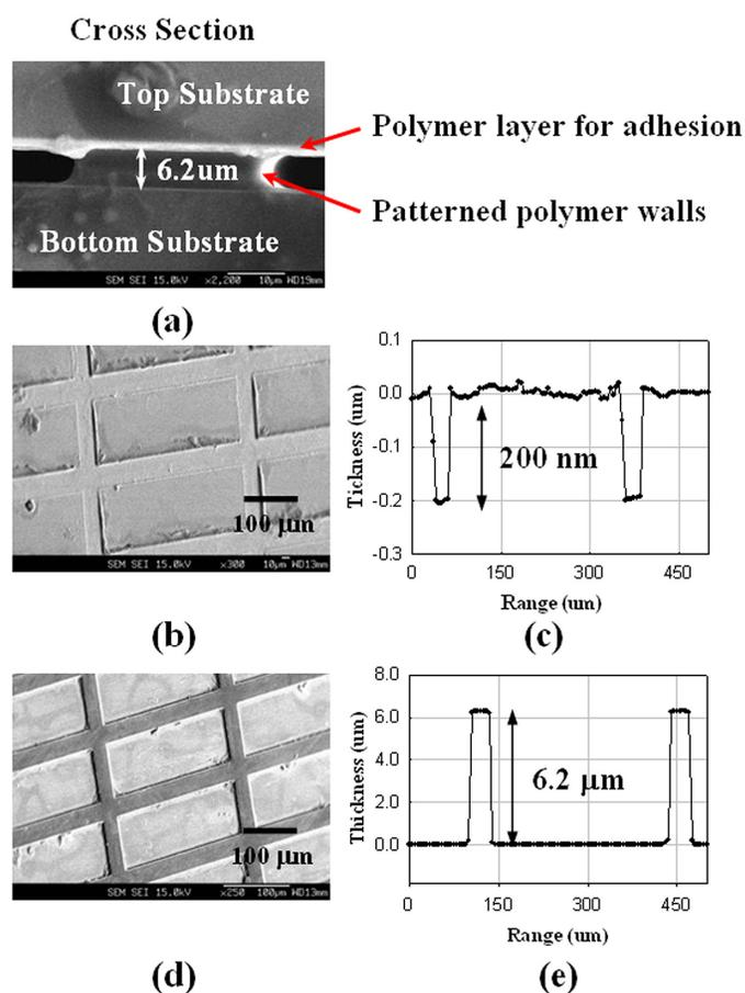
**FIGURE 4** — (a) Cross-sectional SEM image. (b) and (d) are SEM images of the top and bottom surfaces, respectively, observed after separating two substrates, and (c) and (e) are their surface profiles.
