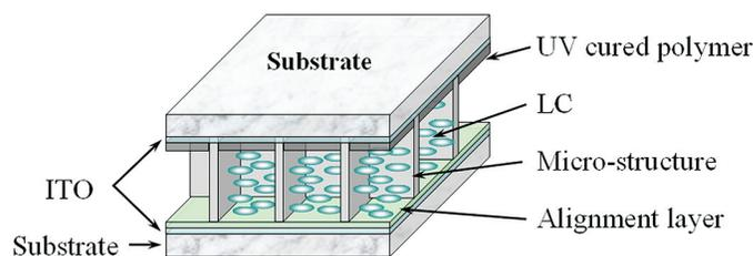
**FIGURE 1** — Schematic diagram of a PILC structure made by patterned microstructures.
