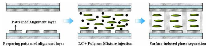
**FIGURE 6** — The schematic diagram of a PILC mode where phase separation is induced by surface-wetting properties.
