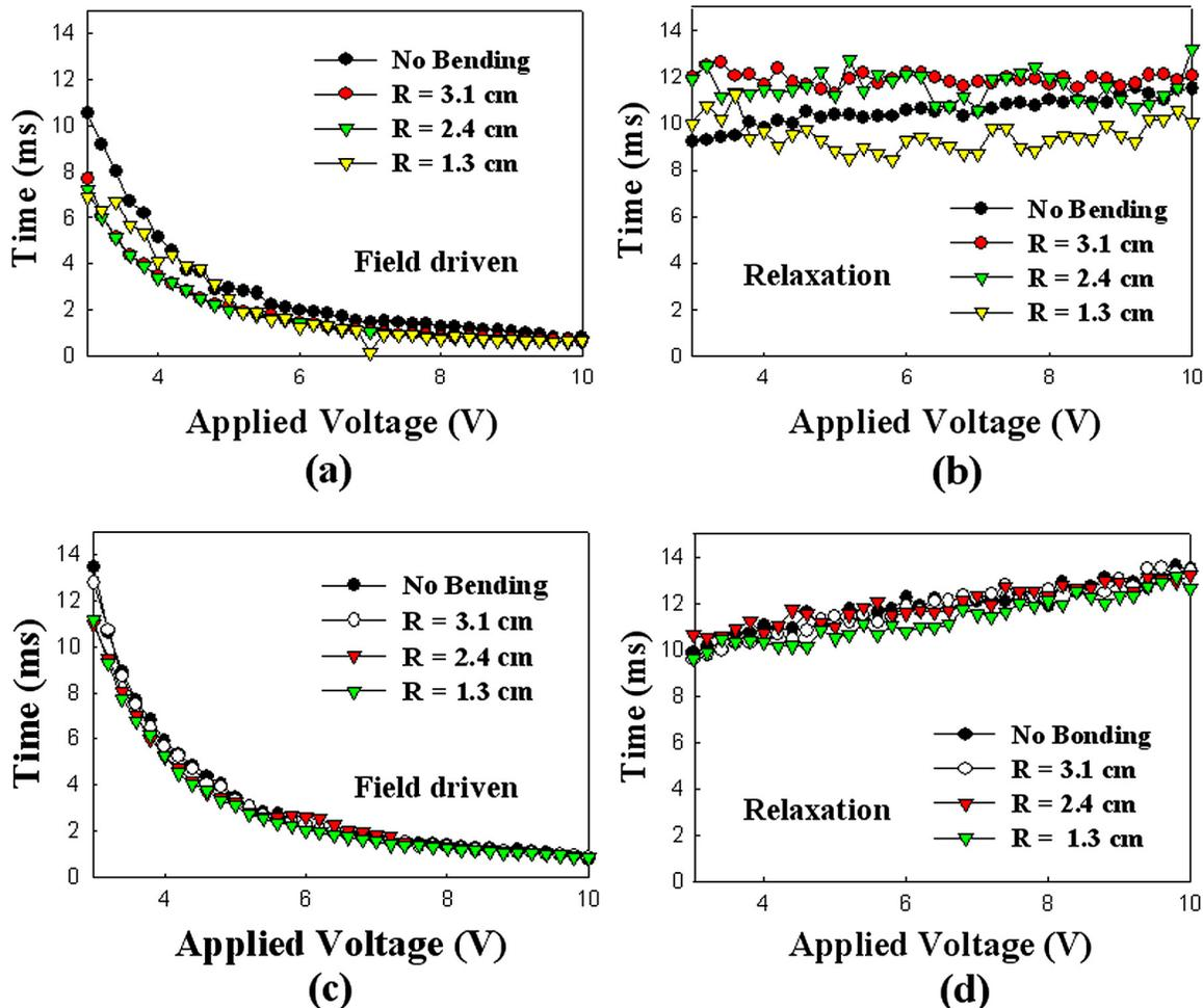
**FIGURE 10** — Dynamic properties of field-driven and field-off relaxation times for a normal sample [(a) and (b)] and a PILC sample [(c) and (d)] depending on the degree of bending.
