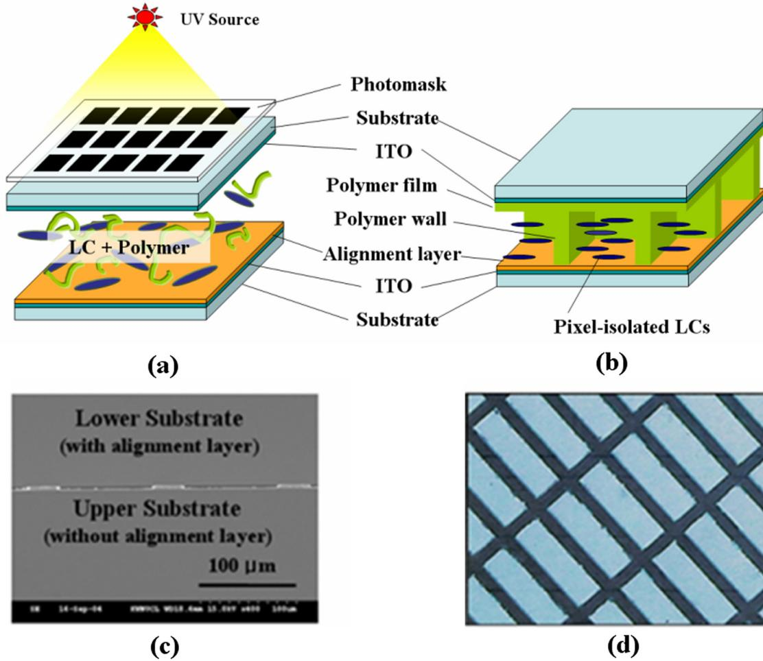
**FIGURE 5** — (a) Schematic diagram of PILC mode made by photo-polymerization-induced anisotropic phase separation, (b) pixel structure after UV exposure, (c) the cross-sectional SEM image of PILC sample, and (d) the polarizing optical microscopic texture of the PILC cell.
