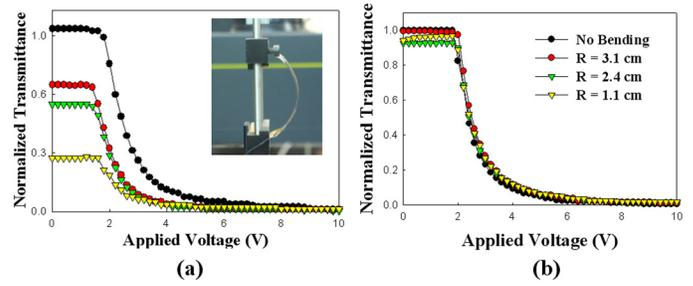
**FIGURE 9** — EO properties of (a) a normal and (b) a PILC sample depending on the degree of bending.
