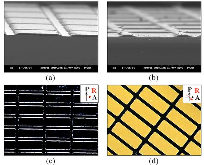
**FIGURE 3** — (a) and (b) are SEM images of the micropatterned SU-8 master substrate and the stamped PDMS structure, respectively. (c) and (d) are polarizing microscopic textures of the PILC cell obtained when the rubbing direction of the sample is parallel and  $45^{\circ}$ -rotated with respect to the polarizer in the absence of an applied voltage, respectively.
