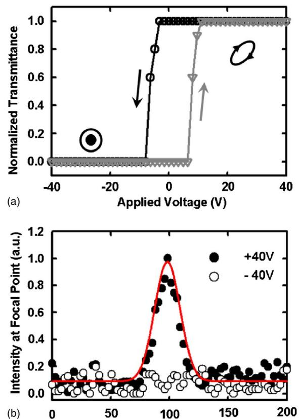
FIG. 4. (Color online) (a) Transmittance of the FLC device under crossed polarizers as a function of an applied voltage. Inserted figures are the polarization states entering the LCP MLA. (b) The intensity profiles of the FLC device. Symbols denote the experimental data and line is the Gaussian fit.
