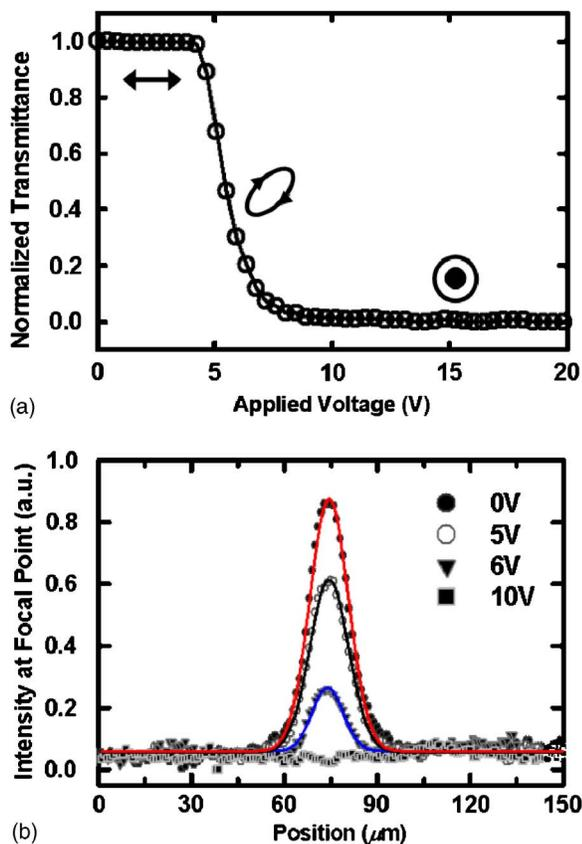
FIG. 3. (Color online) (a) Transmittance of the TN device under crossed polarizers as a function of an applied voltage. Inserted figures represent the corresponding polarization states after passing the TN LC layer. (b) The intensity profiles of the single spot at the focal plane. Symbols denote the experimental data and lines are the fitted results for Gaussian function.
