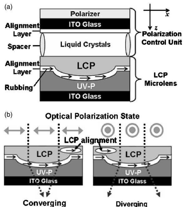
FIG. 1. (a) Schematic illustration of device configuration. (b) Polarization sensitive operations of the LCP microlens.
