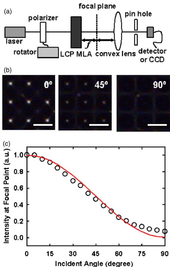
FIG. 2. (Color online) Characteristics of the LCP MLA. (a) Experimental setup for measuring a focal property. (b) Charge coupled device captured images of the LCP MLA at the focal plane. The incident angles with respect to the  $x$  axis are denoted. Scale bar is  $200 \mu\text{m}$ . (c) Intensity of one spot at the focal plane as a function of the azimuthal angle of the incident linearly polarized light.
