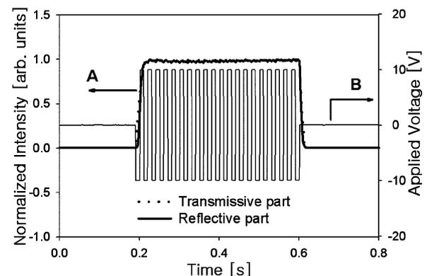
Fig. 6. EO response time of developed transfective LCD. Lines A and B are the normalized EO response and the input pulse, respectively.
