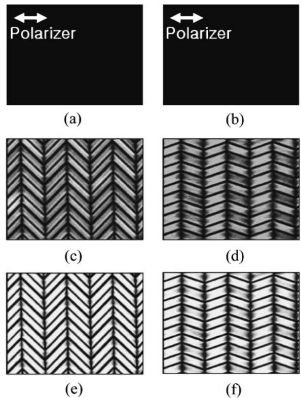
Fig. 4. Polarizing microscopic images of developed transfective LCD. (a), (c), and (e) are textures at applied voltages of 0, 4, and 11 V in transmissive part, respectively. (b), (d), and (f) are textures at reflective part at the same applied voltages.
