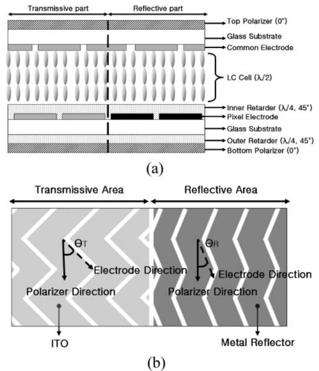
Fig. 1. Schematic diagram of proposed transflective LCD: (a) cross-sectional structure and (b) pixel electrode configuration of bottom substrate in transmissive and reflective parts.
