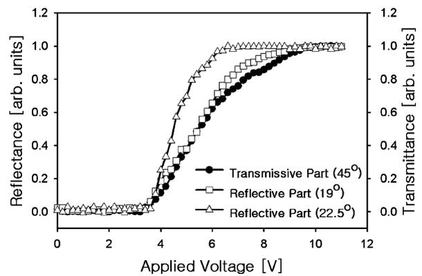
Fig. 5. Measured EO characteristics of developed transfective cell.
