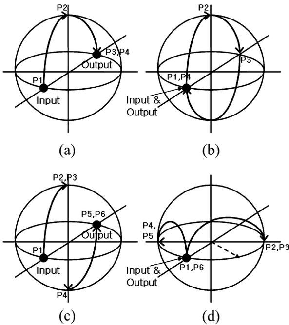
Fig. 2. Poincare sphere representation of polarization path of (a) dark and (b) bright states in transmissive part, and (c) dark and (d) bright states in reflective part.
