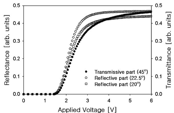
Fig. 3. Simulated EO characteristics of developed transfective cell for various patterning angles.
