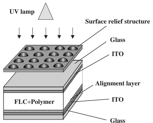
Fig. 1. Schematic diagrams of fabrication setup of nematic LC microlens array. The surface relief array of hemisphere is fabricated using UV-curable polymer.
