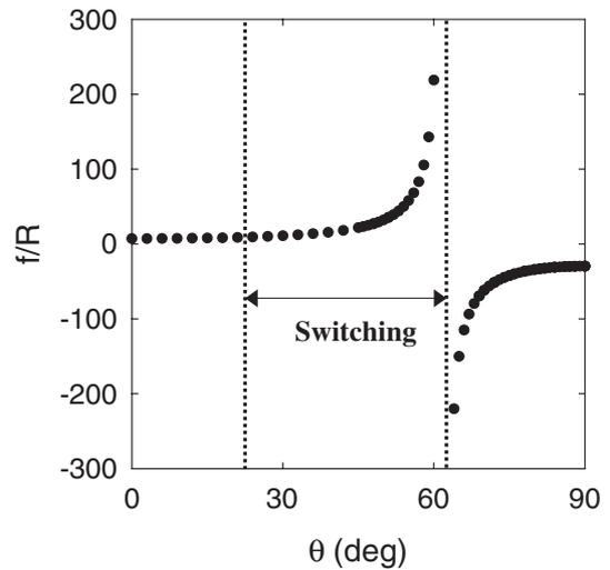
Fig. 3. Calculated focal length as a function of smectic tilt angle  $\theta$  using eqs. (1) and (2) (see text). The tips of the arrows indicate the two stable operating states shown in Fig. 2(b).
