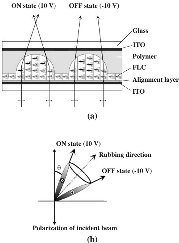
Fig. 2. Schematic diagrams of (a) light propagation through FLC microlens structure and (b) orientation of FLC molecules in two states in the  $x$ - $y$  plane as viewed along the direction normal to the cell.
