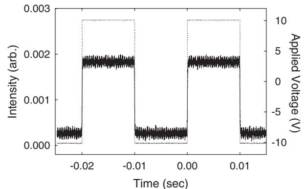
Fig. 6. Transmission vs time curve for FLC microlens. ON and OFF times are 150 and 88  $\mu\text{s}$ , respectively.
