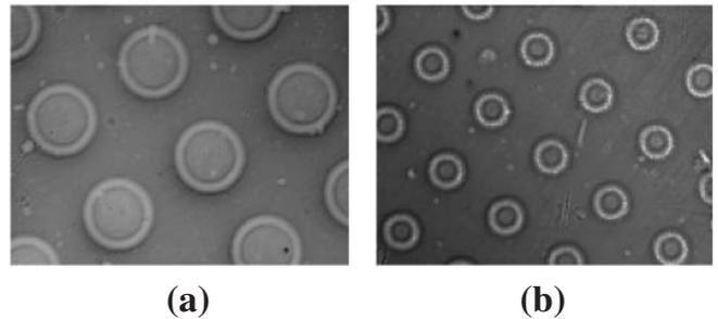
Fig. 4. Microscopy image of two microlens arrays, with lens diameters of (a) 355  $\mu\text{m}$  and (b) 225  $\mu\text{m}$ , as viewed through a polarizing microscope without any applied voltage.
