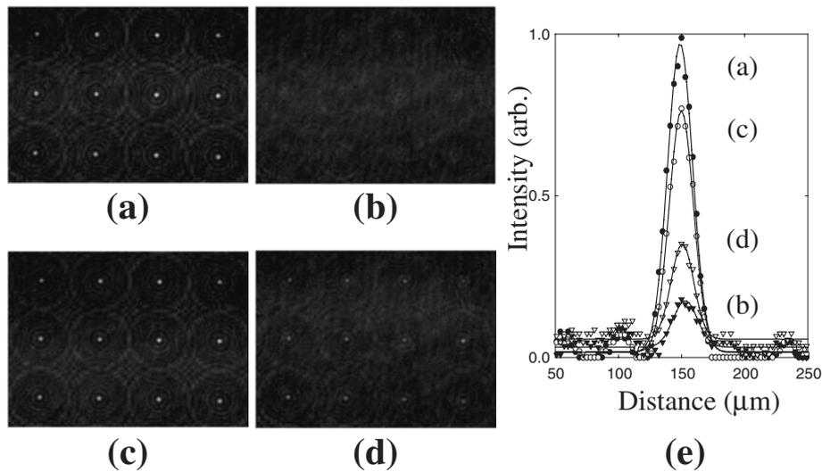
Fig. 5. Focusing characteristics of microlens for laser beam passing through lens 355  $\mu\text{m}$  in diameter. (a) and (b) are beam images at 11 mm with +10 and  $-10$  V, respectively. Panels (c) and (d) show the images of the beam when the applied voltage is changed from +10 to 0 V and  $-10$  to 0 V, respectively. (e) Profiles of transmitted light beam in (a) and (d).
