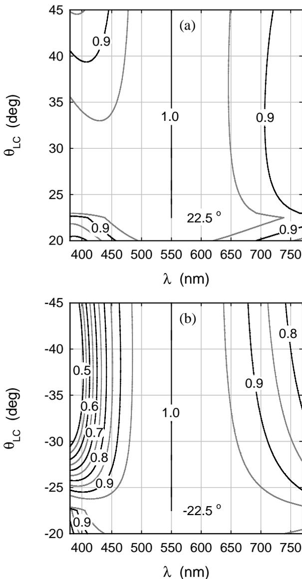
Fig. 4. Iso-reflectance curves for the two in-plane optical geometries as a function of the wavelength ( $\lambda$ ). The calculations were performed along the maximum reflectance line obtained with fixed wavelength of 550 nm.
