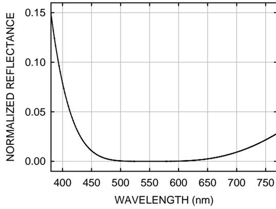
Fig. 2. Optical dispersion of the reflectance in the range of visible light for normal incidence when the optic axis of the LC layer is parallel to the polarizer.
