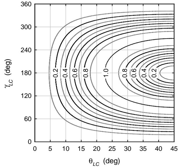
Fig. 3. Iso-reflectance curves given in the plane of the molecular rotation or the rotation of the average optical axis ( $\theta_{\text{LC}}$ ) and the phase retardation ( $\gamma_{\text{LC}}$ ) of the LC layer for normal incidence.
