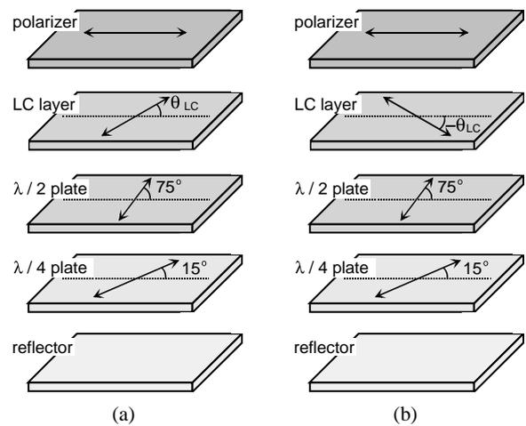
Fig. 1. Two in-plane optical geometries of a reflective LCD: (a) the counter-clockwise rotation and (b) the clockwise rotation of the average optic axis of the LC layer. A combination of the HW and QW plates is used for the WQ plate.
