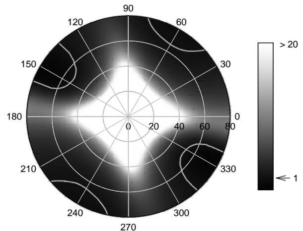
Fig. 5. Gray scale representation of the iso-contrast map for a reflective LCD cell with  $\theta_{\text{LC}} = -22.5^\circ$ . The white solid curves represent the inversion lines of contrast.
